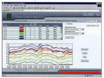
Internet-based SCADA systems enable operators to access real-time and historical data, such as exhaust temperature trends, from anywhere in the world.
