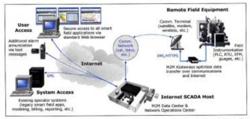
Internet-based SCADA systems can reduce the cost and complexity of long-distance communications, because each piece of remote equipment is connected to an Internet Point of Presence (IPP or ISP).
